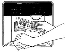
Do not pour water in spill shelf because it is not self-draining pour it in kitchen sink. The shelf and its grille should be cleaned regularly according to instructions on page 18.
